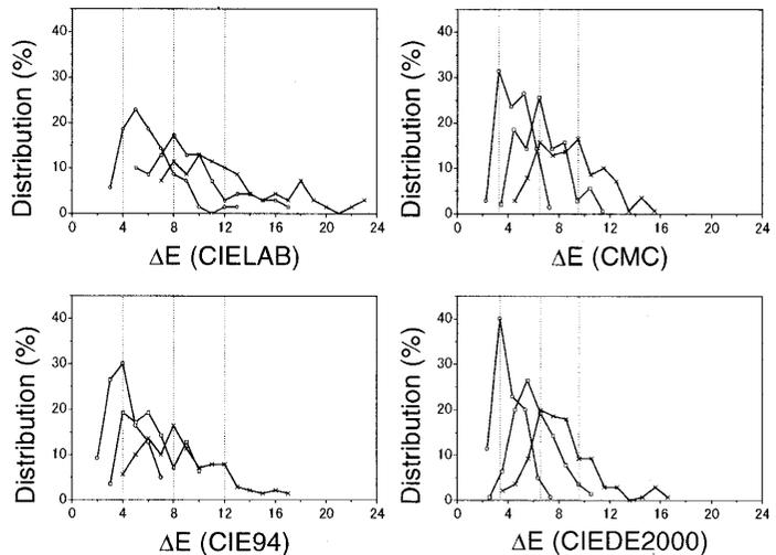
FIG. 11. Distribution of color pairs, in percentage of the total pairs, predicted to scatter in the successive intervals of 1  $\Delta E$  unit across the whole data set by individual color-difference formulas. The dotted vertical lines indicate the predicted color differences corresponding to the three reference visual scales of 4.0 (○), 8.0 (□), and 12.0 (×) CIELAB  $\Delta E$  units, respectively.
