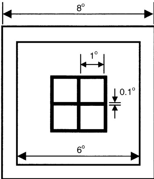
FIG. 1. The test stimulus arrangement used in color discrimination threshold experiment. A four-square array, with  $0.1^\circ$  separation and frame, was presented on a  $6^\circ$  background of the center color, surrounded by a bright border of  $8^\circ$  visual angle, out of which was a black screen. See text for details.
