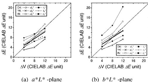
FIG. 9. Visual data, as in Fig. 6, for the  $L^*$  axis in the CIE green center: (a)  $a^*L^*$  plane, (b)  $b^*L^*$  plane.
