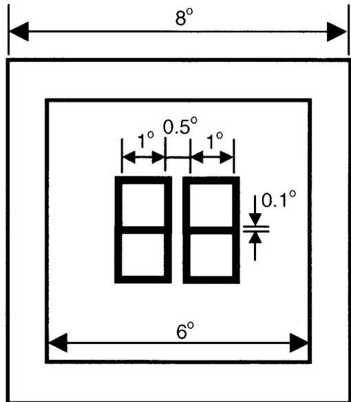
FIG. 2. The test stimulus paradigm used in the color-difference comparison experiment. The construction was almost the same as that in Fig. 1, except that two color pairs were presented at the center of the background, whose color was set as Munsell N5 instead of the test center color. See text for details.
