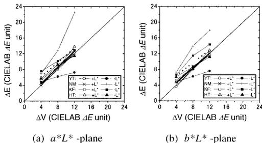
FIG. 6. Relation of visual and colorimetric scales in CIELAB  $\Delta E$  units for  $L^*$  axis at the CIE gray center: (a)  $a^*L^*$  plane, (b)  $b^*L^*$  plane.
